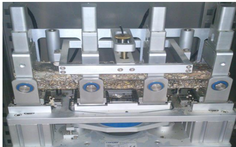
Figure 1. Four-Point Flexural Bending Beam Test Setup
