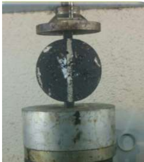
Figure 4. Indirect Tensile Strength Test Setup
