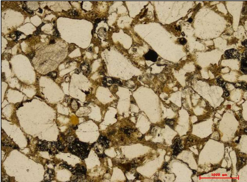
**Figure 9.** Mortar's examination by polarizing microscope (Analyzer absence)
