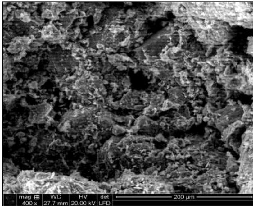
**Figure 2.**Mud brick's sample examination with SEM (mag 400×)
