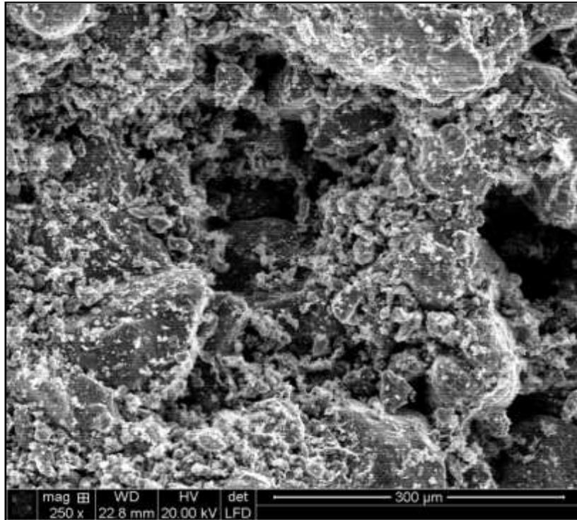
Figure 3. Mortar's sample examination with SEM (mag 250×)
