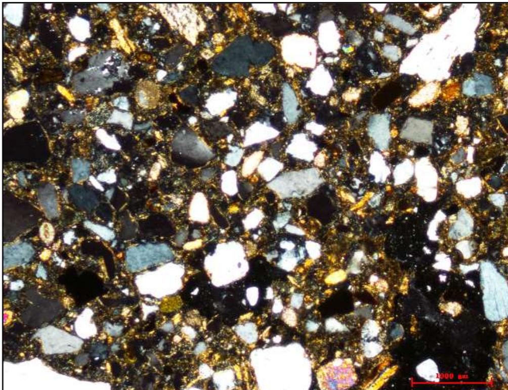
Figure 6. Mud brick's examination by polarizing microscope
