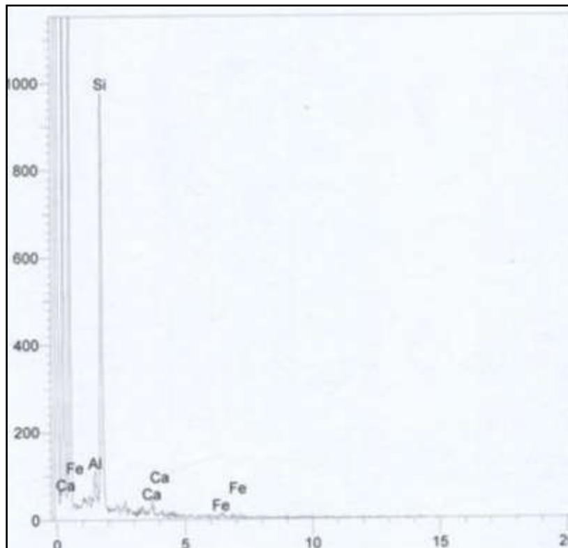
Figure 4. EDAX analysis of mud brick's sample
