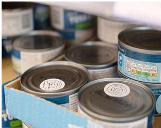
**Figure 8.** NFC-enabled smart stickers carry the Provenance mark along with item or batch IDs.
